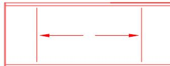
Fixed glass both ends with opening glass opening in both directions.
