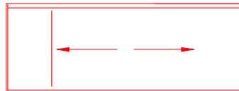
Fixed glass one end with opening glass opening in both directions.
